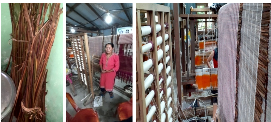
A weaving unit in North Sikkim making mats from large cardamom pseudo-stem fibres
