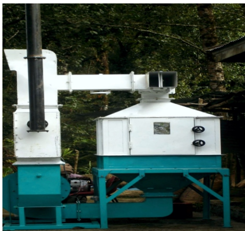
Dryer run on Electricity/diesel or both
