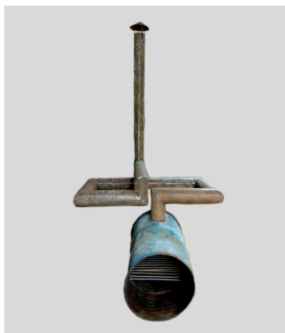
Flue pipe with furnace
